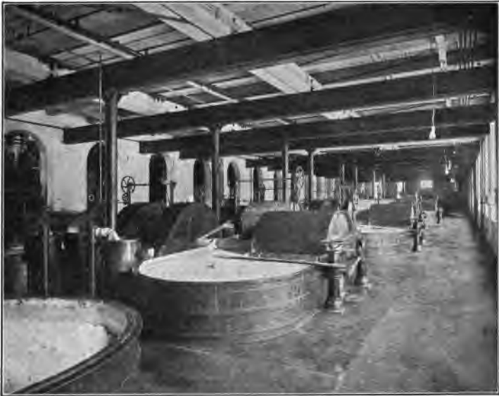
FIG. 136.—The beaters which convert the rags into pulp. (Courtesy of B. D. Rising Paper Co.)
